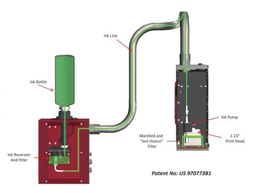
The head can be changed in the field without disassembling the ink delivery system and or any of the ink delivery connections. The system can be installed, primed and operational in less than 1 hour.
